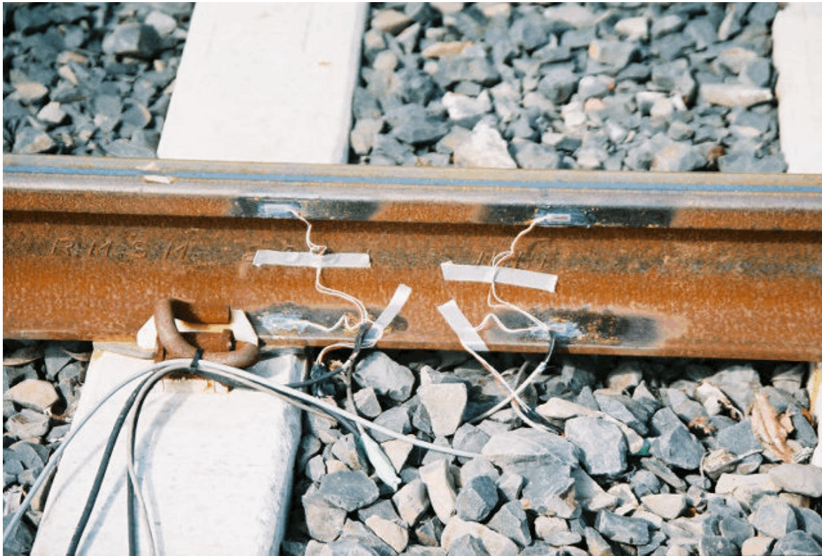
FIGURE 18 - STRAIN GAGE INSTALLATION AT SITE 1 (FROM 2005 TESTS)
