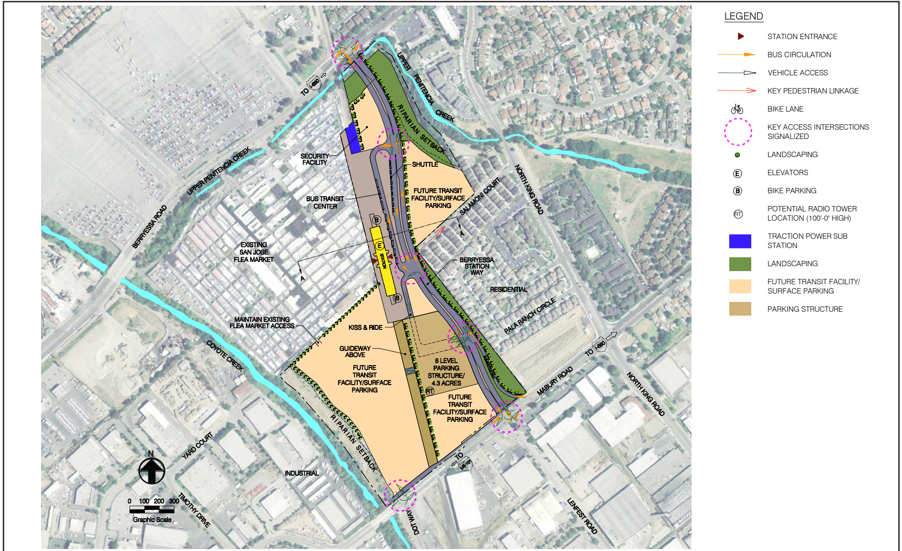
Figure 2-17A: Berryessa Station North Option Conceptual Site Plan – SVRTP Alternative
