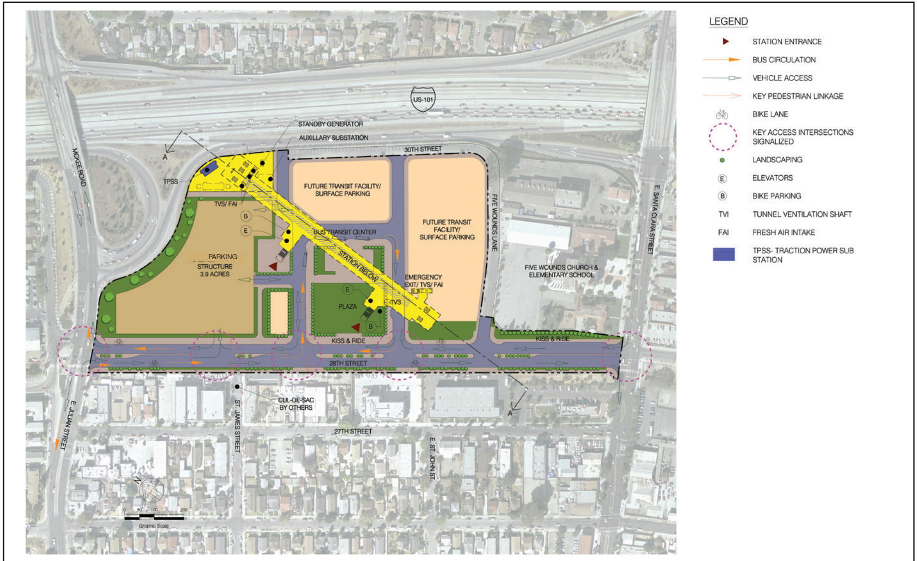
Figure 2-18: Alum Rock Station Conceptual Site Plan
