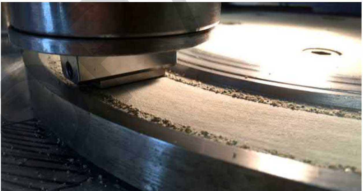
Figure 8. Close up taken during SAT™ testing, showing the test track on the rotating steel disc after the abrasion material has passed under the test piece.
