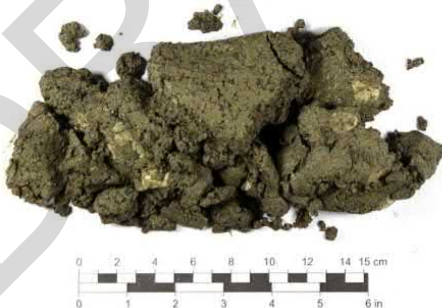
Sample No. 6, marked "BH-116". SAT™ powder was prepared by soft hammer and sieving with steel balls.
