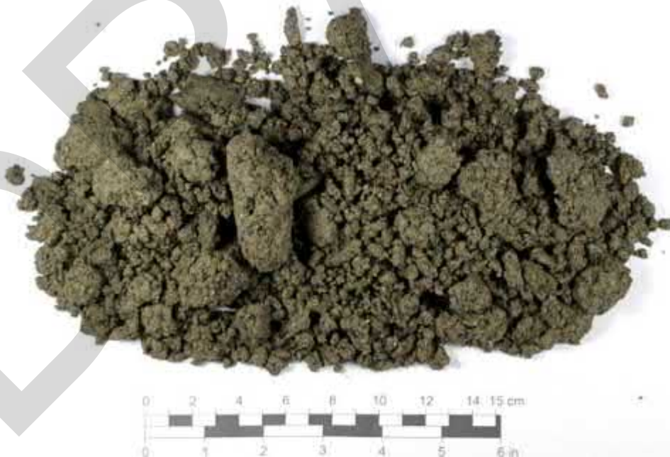
Sample No. 4, marked "BH-112" SAT™ powder was prepared by soft hammer and sieving with steel balls.
