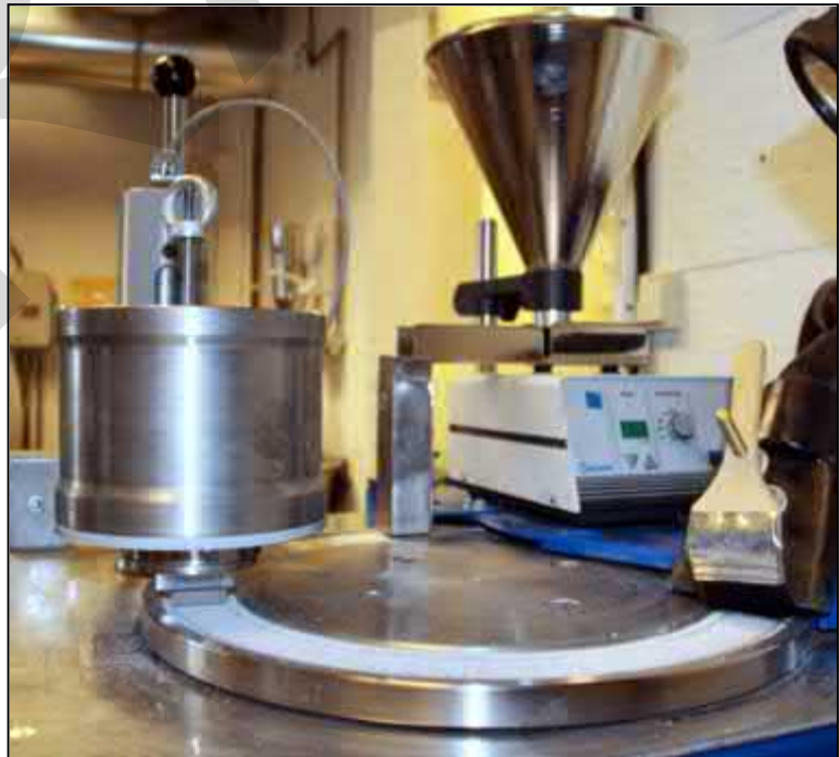
Figure 4. Photos of test equipment used to determine Abrasion Value Cutter Steel (AVS) and Soil Abrasion Test (SAT™).
