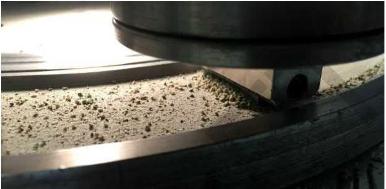
Figure 7. Close up taken during SAT™ testing, showing the test track on the rotating steel disc before the abrasion material has passed under the test piece.
