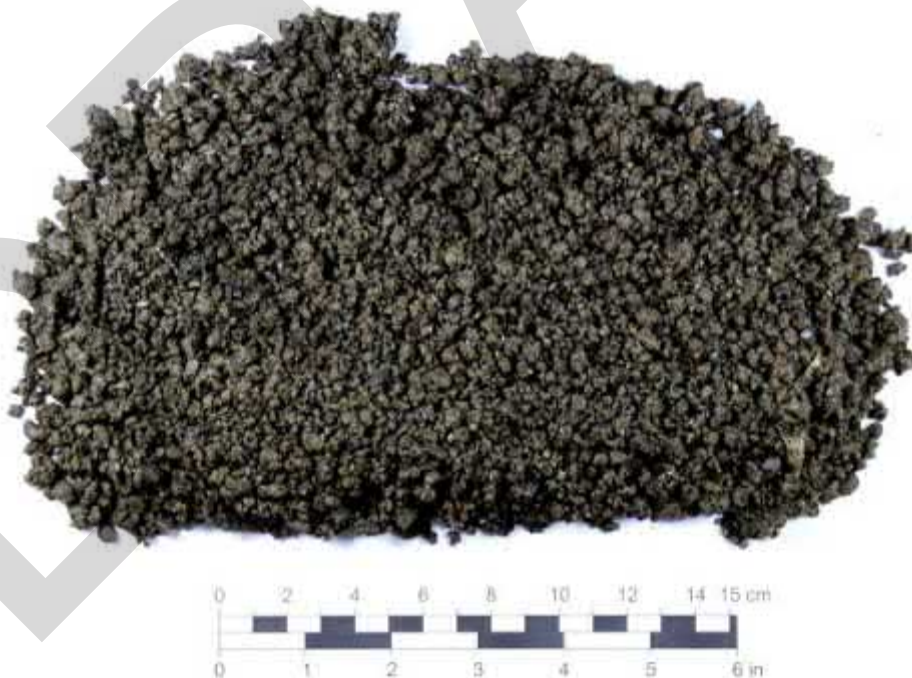
Sample No. 2, marked "BH-141". SAT™ powder was prepared by soft hammer and sieving with steel balls.
