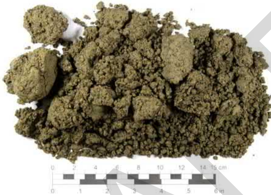
Sample No. 3, marked "BH-124" SAT™ powder was prepared by soft hammer and sieving with steel balls.
