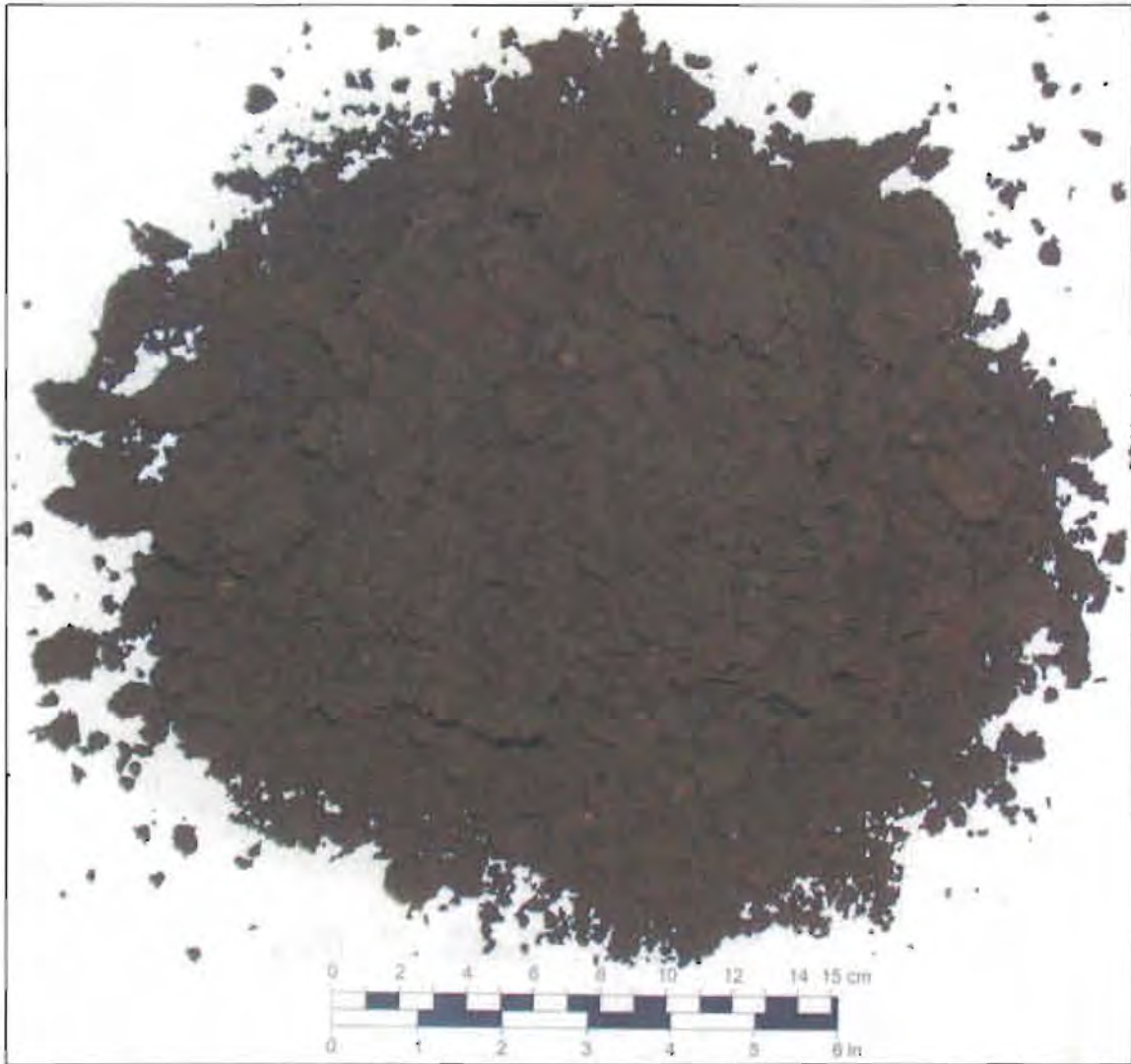
Sample No. 2, BH-31/S-4. SAT powder was prepared by sieving with steel balls. Of the total sample volume, 92.6 % was < 4 mm and 81.7 % was < 1.0 mm after preparation.
