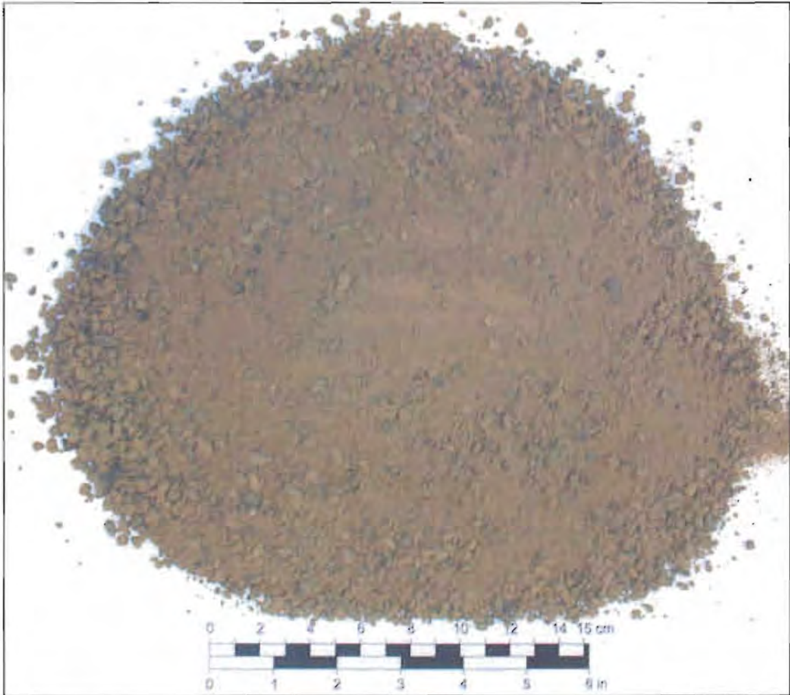
Sample No. 4, MW-8B. SAT powder was prepared by sieving with steel balls. Of the total sample volume, 91.1 % was < 4 mm and 51.9 % was < 1.0 mm after preparation.
