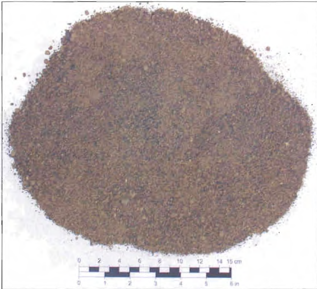
Sample No. 3, MW-61. SAT powder was prepared by sieving with steel balls. Of the total sample volume, 99.1 % was < 4 mm and 84.7 % was < 1.0 mm after preparation.
