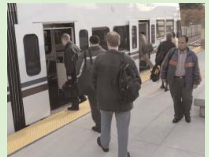
Example of level boarding for a light rail vehicle
