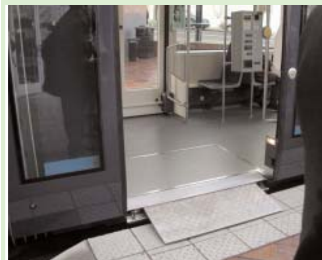
Example of level boarding with a bridge plate
