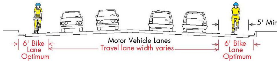
Figure 7-1b: Bike Lane Width - 35-40 mph Posted Speed
