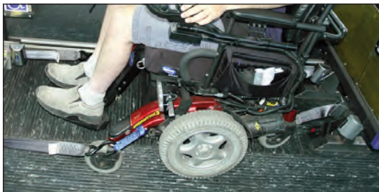
Each bus operator must secure mobility devices, or verify proper securement (secured to the floor) if performed by a passenger or attendant.
