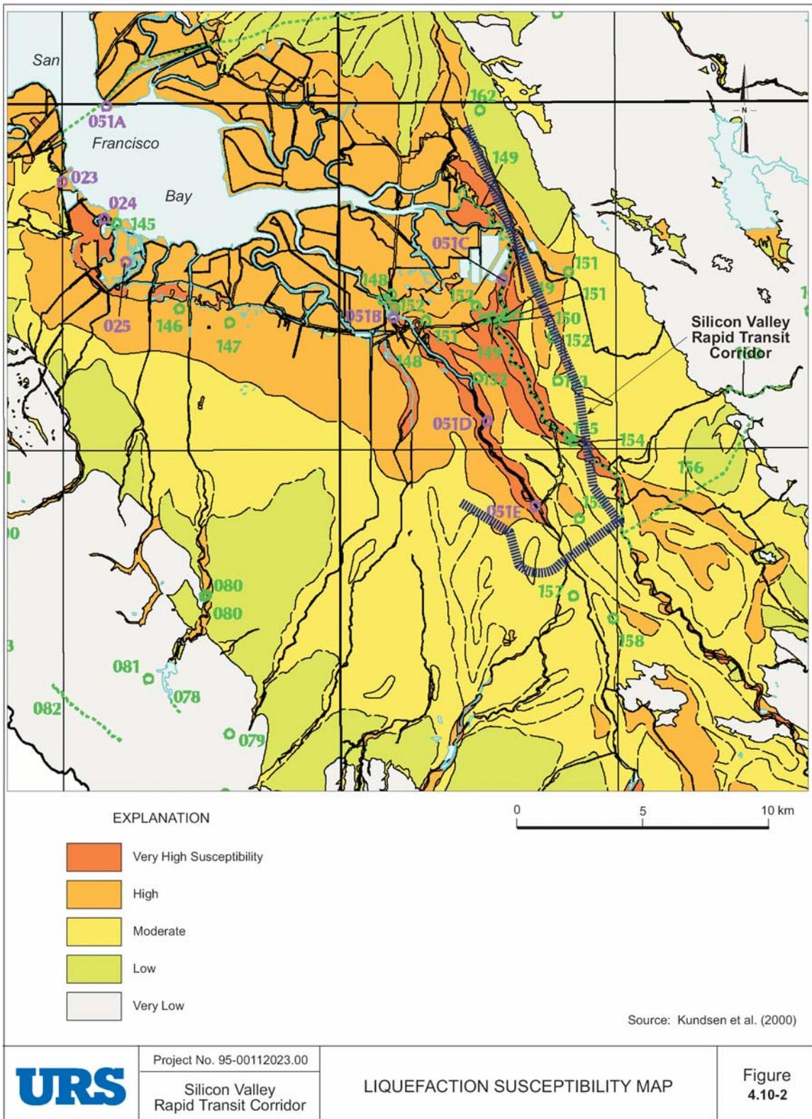
Figure 4.10-2: Liquefaction Susceptibility Map
