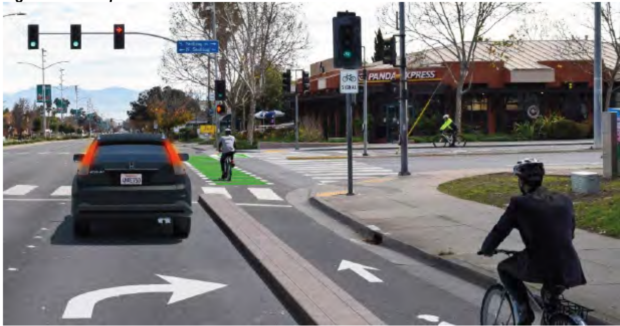
Figure 45. Example of Protected Bike Lanes
