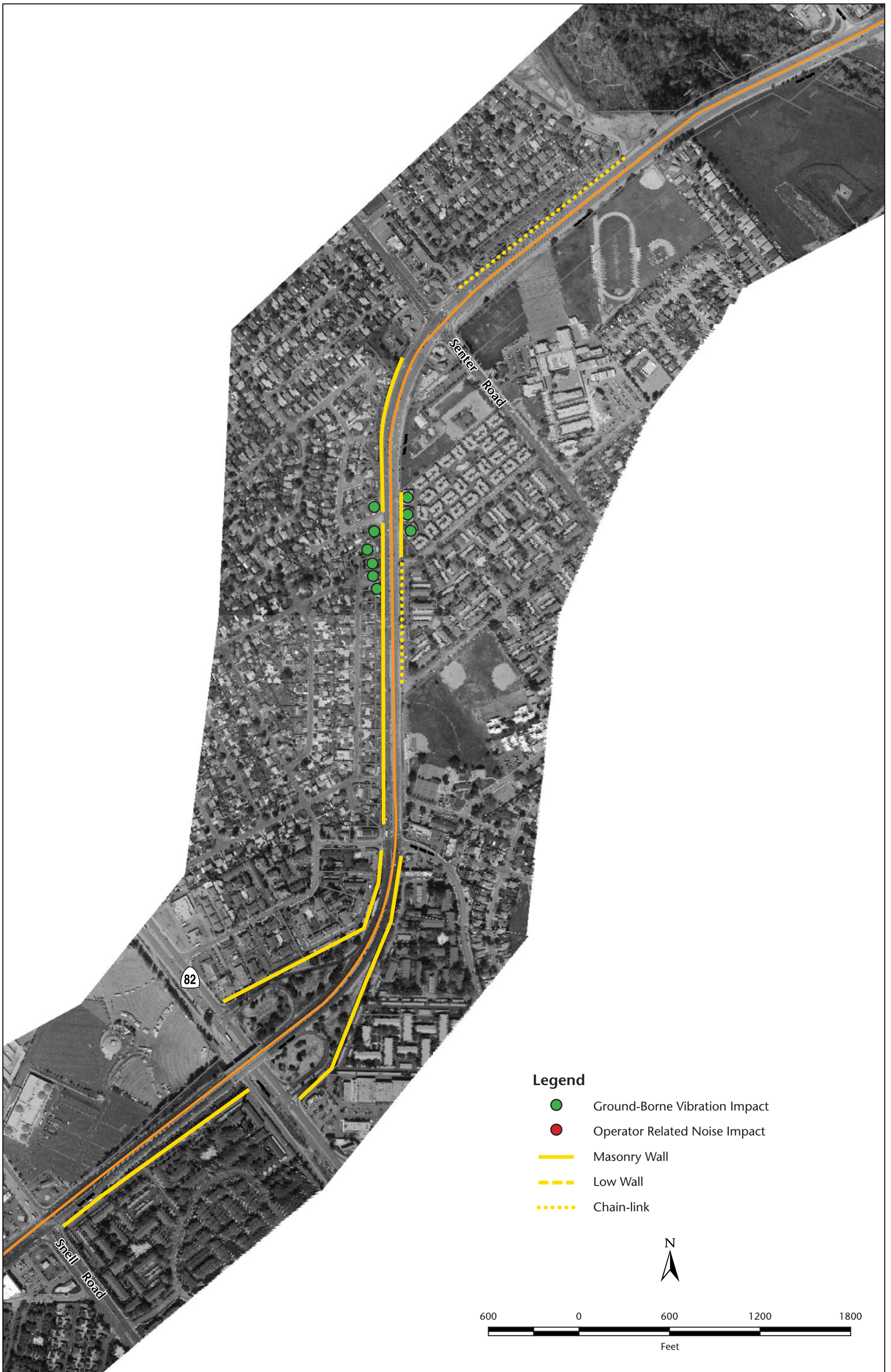
Figure 4.14-5d Locations of Noise and Vibration Impacts and Existing Community Walls for the Light Rail Alternative
