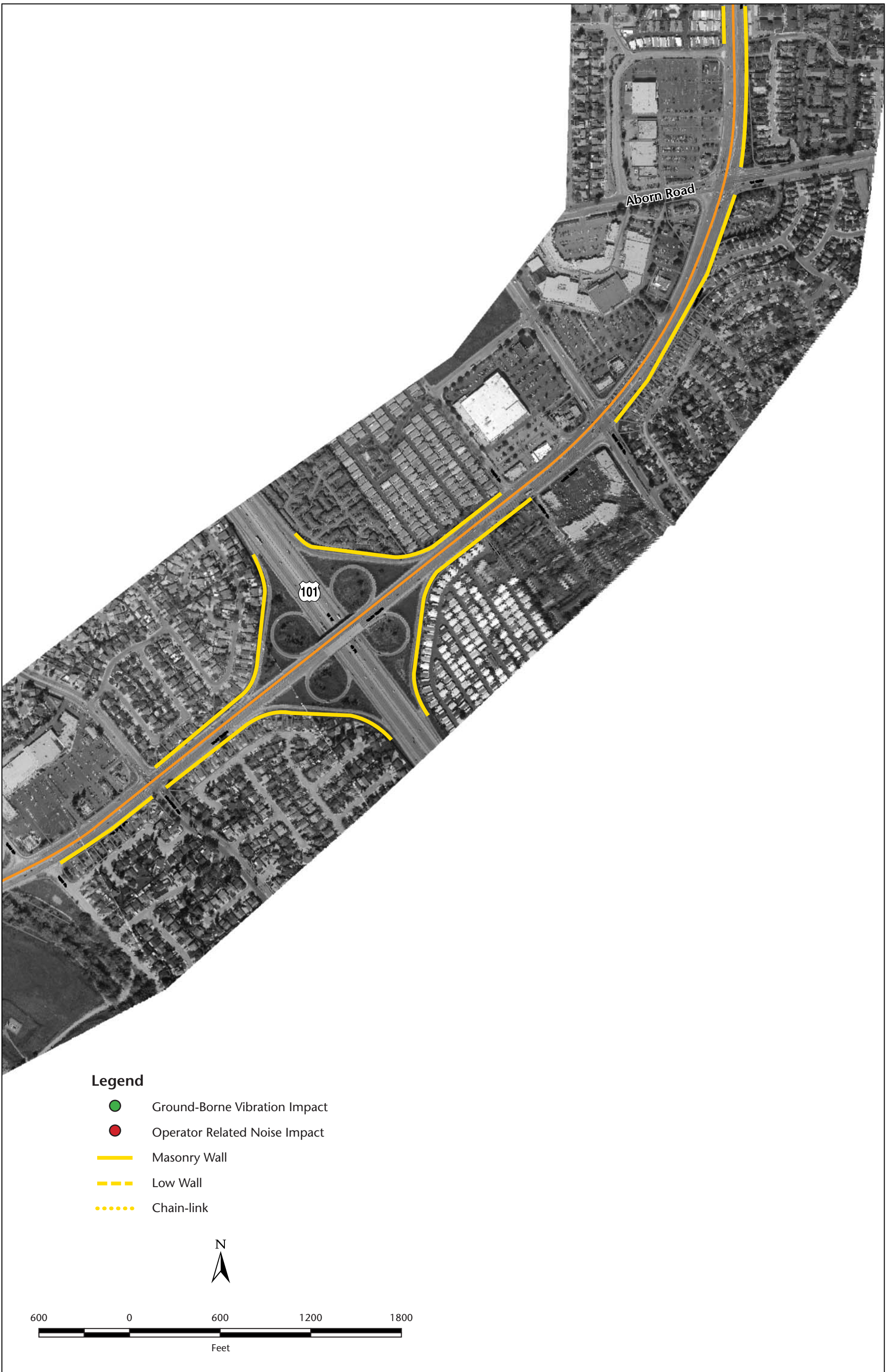
Figure 4.14-5c Locations of Noise and Vibration Impacts and Existing Community Walls for the Light Rail Alternative
