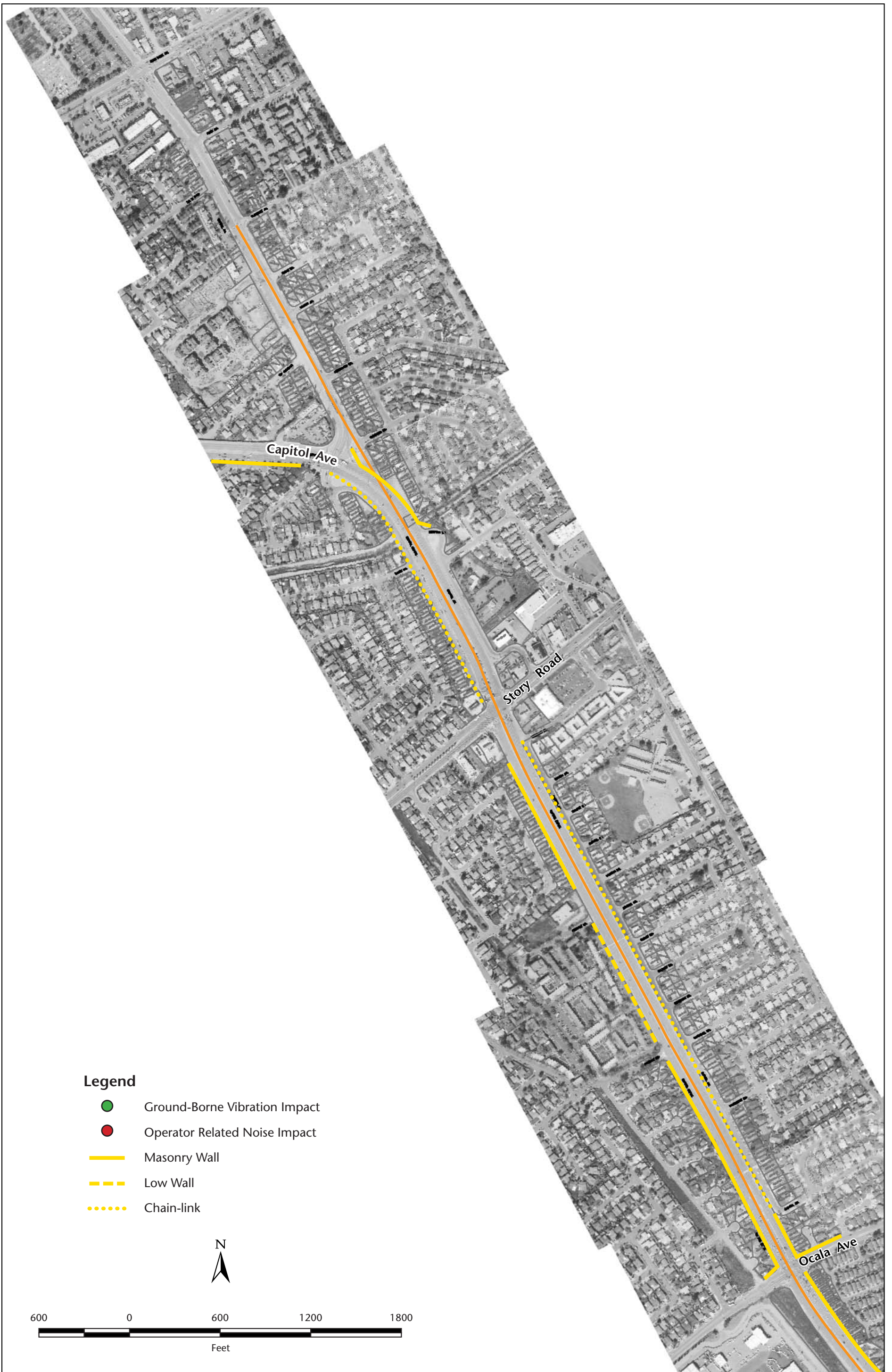
Figure 4.14-5a Locations of Noise and Vibration Impacts and Existing Community Walls for the Light Rail Alternative
