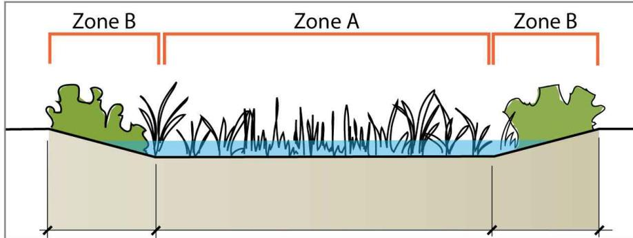
**Uniform surface grade:** This stormwater planter has a flat bottom with consistent depth of ponding across the structure. All of the plants selected for this design must be tolerant of periodic inundation (**Zone A**).
