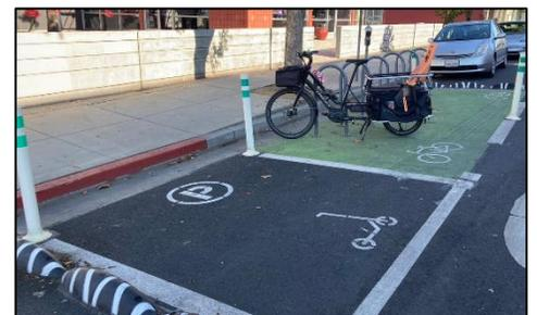
Bike and scooter parking corral replacing an on-street vehicle parking space
