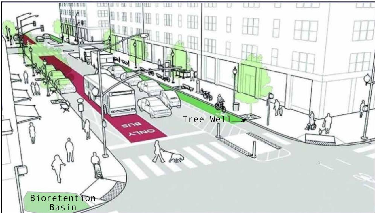
**Figure 2:** Complete Street in Urban Area with tree well and bioretention features
