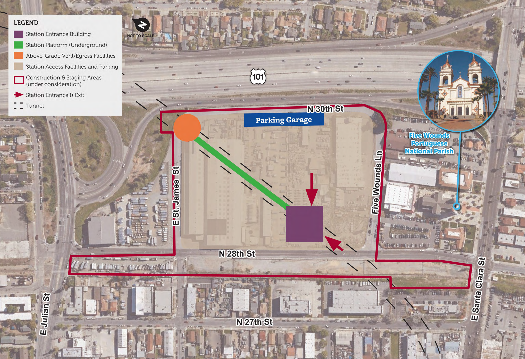
Figure 4: 2024 28th St/Little Portugal Station Conceptual Site Plan VTA's BART Silicon Valley Phase II Extension Project
