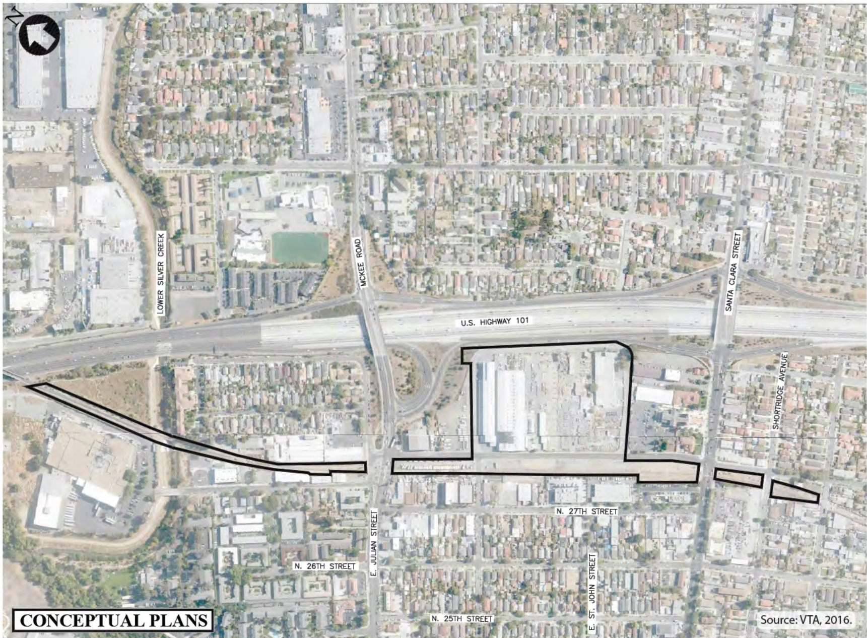
Figure 5-3 Proposed Alum Rock Construction Staging Areas VTA's BART Silicon Valley–Phase II Extension Project
