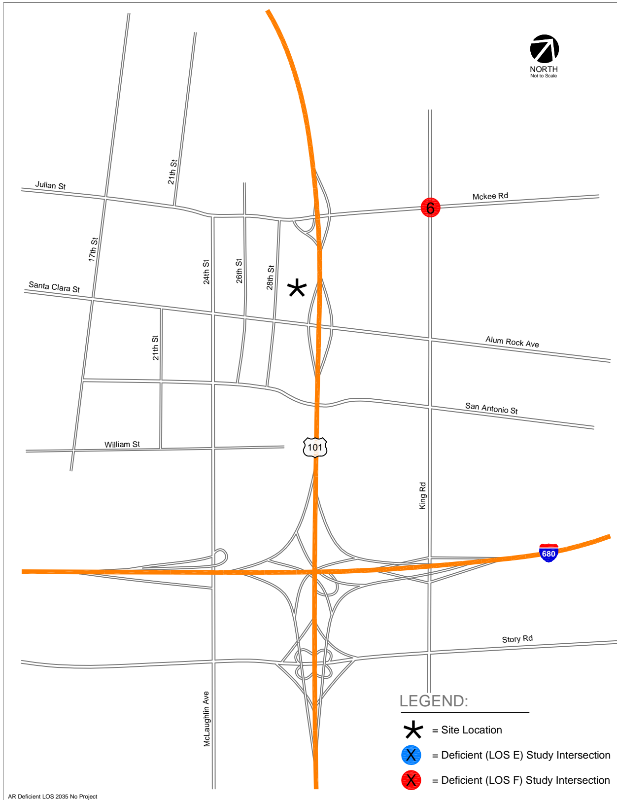
Figure 44 2035 No Project/Phase I Conditions Deficient LOS Intersections – Alum Rock/28 th Street Station
