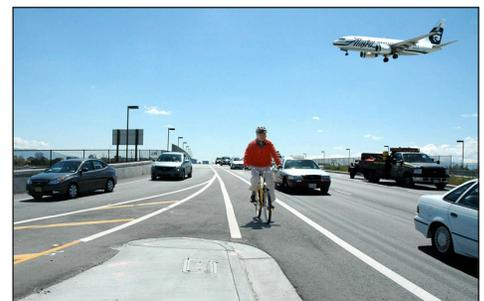
*This bicyclist is correctly positioned in between through and right-turning traffic.*
