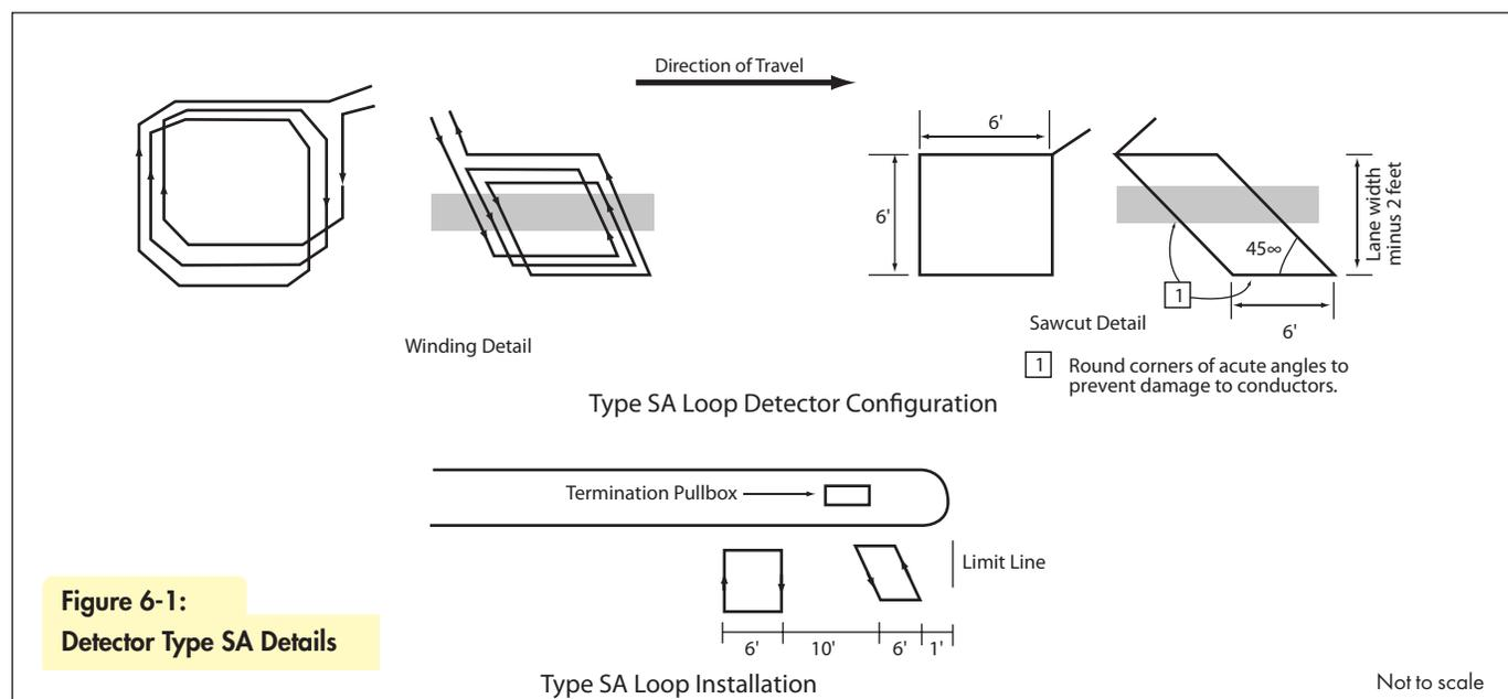
Figure 6-1: Detector Type SA Details
