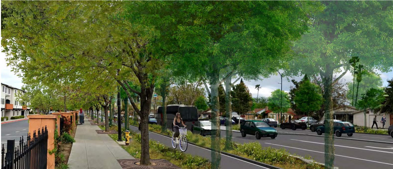
Story Road – This is a typical rendering of the segment improvements on Story Road. Improvements include a widened sidewalk and a street tree and landscape buffer from the separated bikeway. The separated bikeway buffer is widened and includes a landscape median and street trees.
