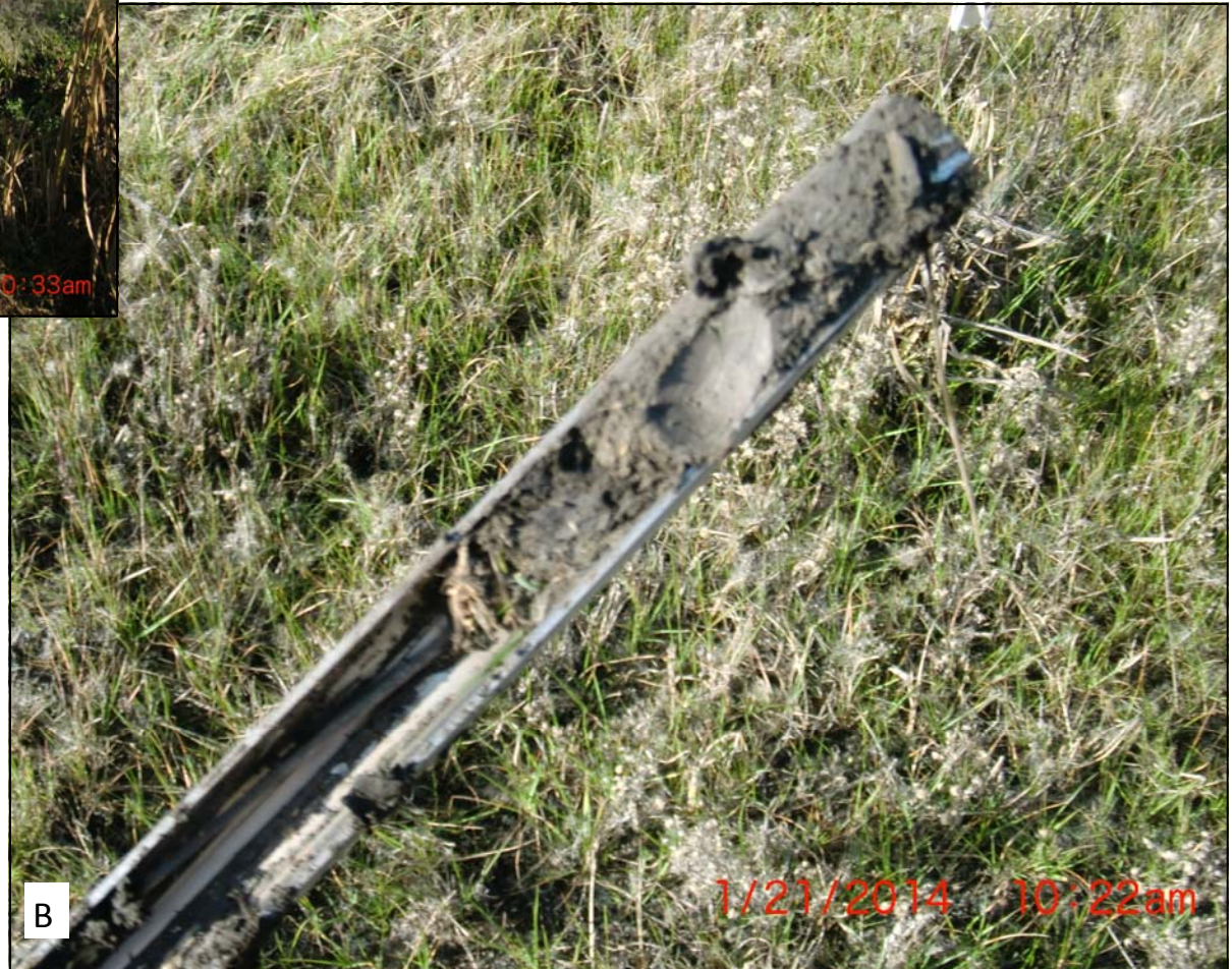
Figure 6. South gage field photos, January 21, 2014. Wrigley Creek Mitigation Performance Monitoring, Santa Clara County, California . Photo A shows ponded water upstream of the south gage, suggesting continually saturated soil during an inter-storm period. This moist soil was directly observed with a soil sampler (Photo B).
