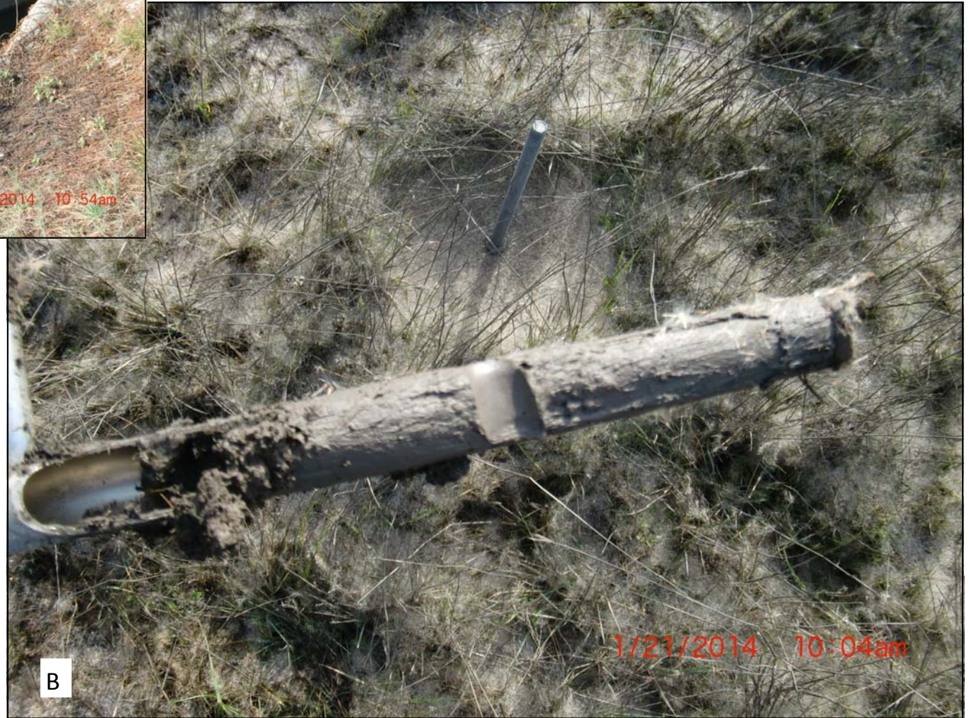
Figure 5. North gage field photos, January 21, 2014. Wrigley Creek Mitigation Performance Monitoring, Santa Clara County, California . Photo A shows ponded water downstream of the north gage at the downstream culvert inlets, which supports continually saturated soil moisture during an inter-storm period. This moist soil was directly observed with a soil sampler (Photo B).
