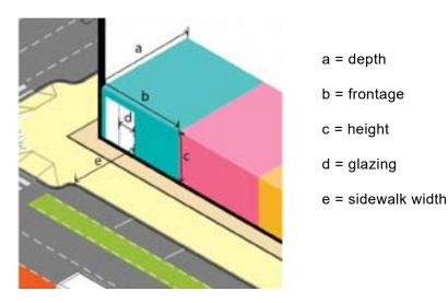
Guidelines for appropriate façade design, ceiling height, shop space depth, utilities, and other elements of building design can help ensure that new space supports a range of commercial uses.
