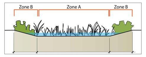
Uniform surface grade: This stormwater planter has a flat bottom with consistent depth of ponding across the structure. All of the plants selected for this design must be tolerant of periodic inundation (Zone A).
