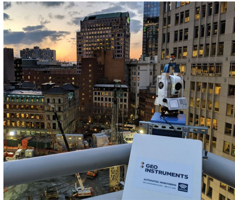
Example of Automated Motorized Total Stations (AMTS), which measures ground movement
