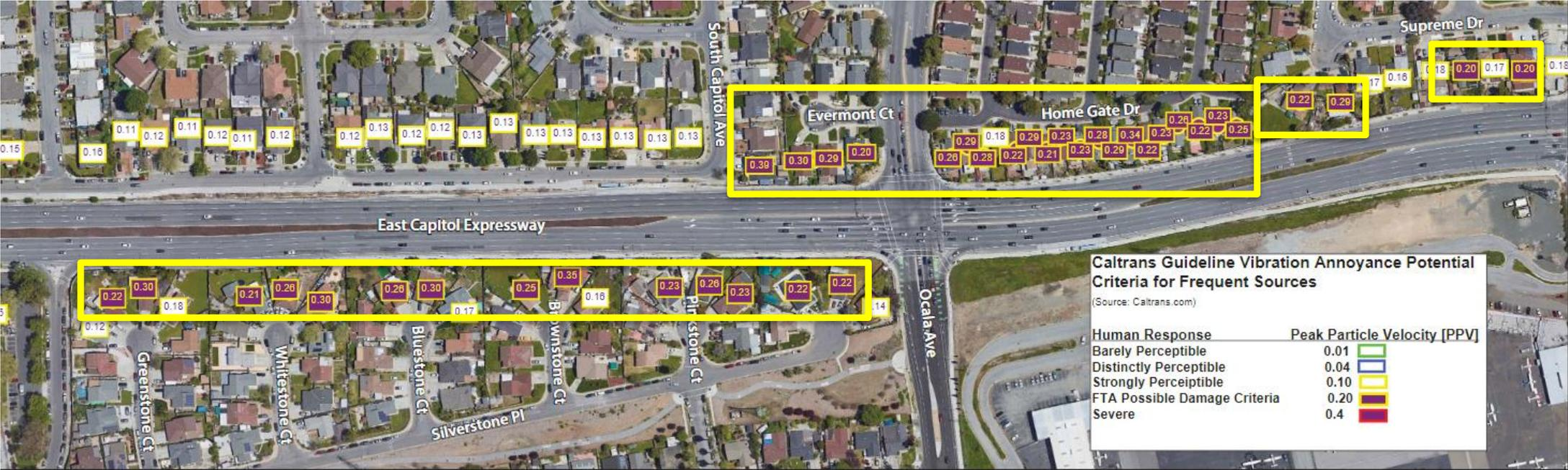
Image showing homes identified as located where vibration could exceed FTA criteria.
