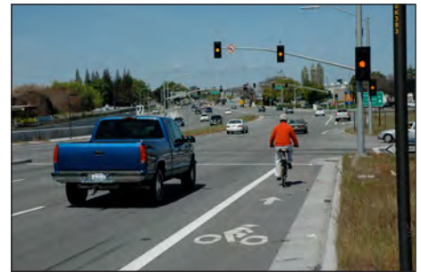
This cyclist may not be able to stop when the light turned yellow and needs the clearance interval to cross to the far side of the intersection.
