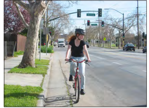
The concrete gutter serves as the comfortable lateral clearance but not essential maneuvering space as defined in Figure 2-1.
