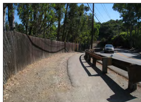
This roadside path in Los Altos Hills is separated from the roadway by a guard rail within the horizontal curve.
