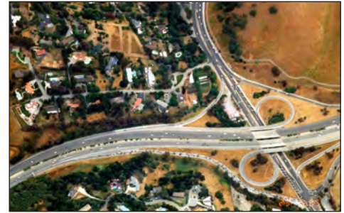
Typical Type L-9 freeway interchange of the 1960's designed with only motor vehicle traffic flow in mind; new and modified partial-cloverleaf interchanges should look like Figure 5-12 instead.
