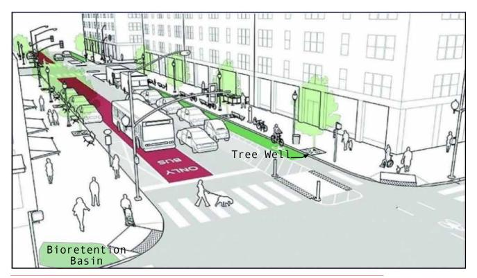
**Figure 2:** Complete Street in Urban Area with tree well and bioretention features Credit: www.vta.org/projects-and-programs/complete-streets
