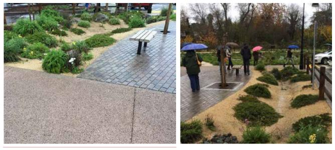
Figure 10: Parking Lot with Runoff Reduction Measures
