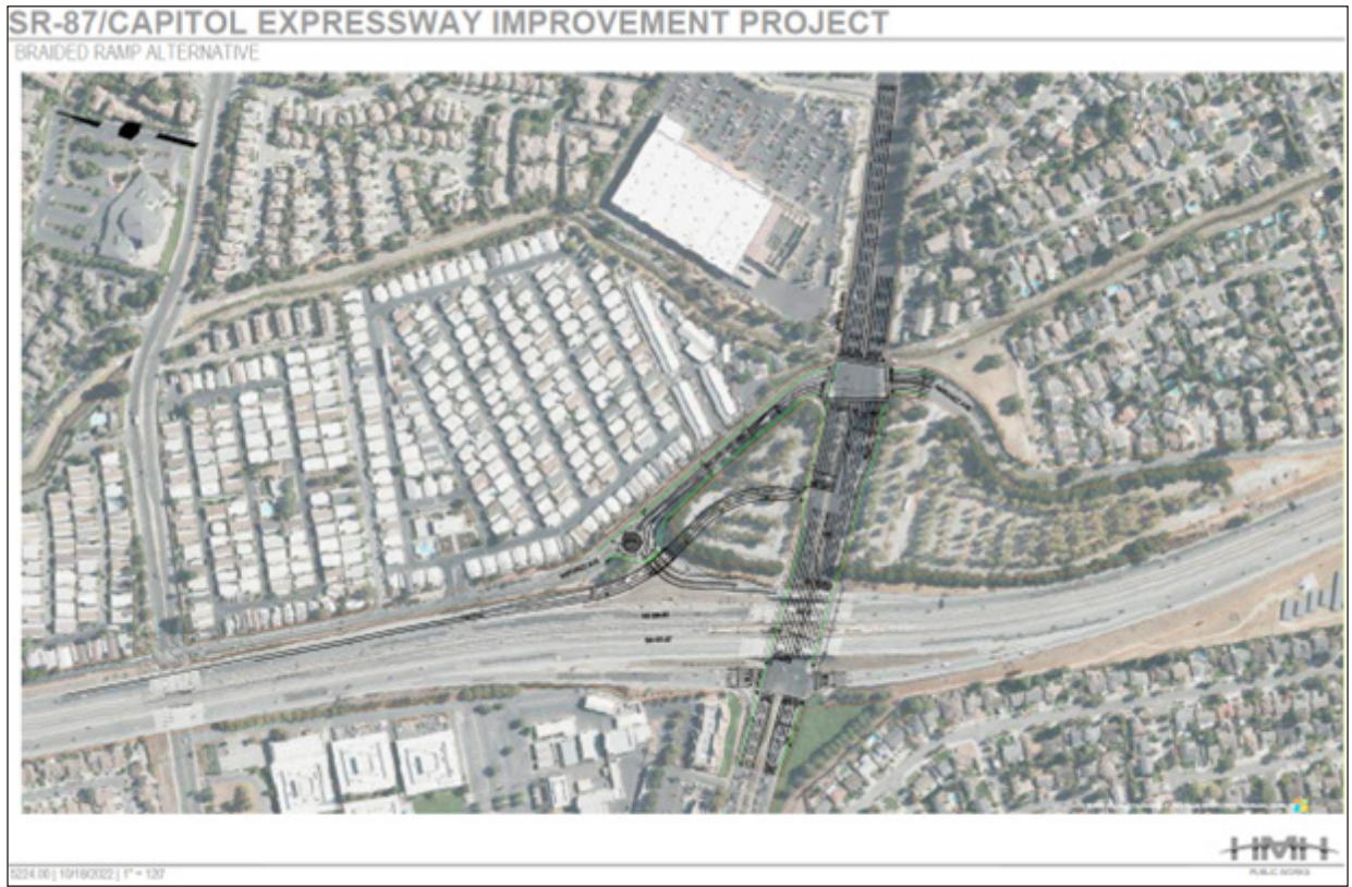
Figure 3.5 Braided Ramp Alternative
