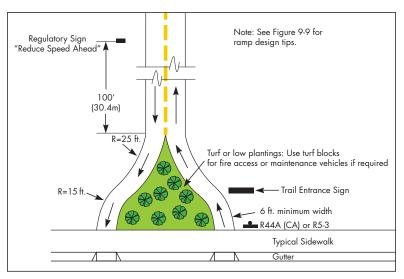
Figure 9-6: Optimal Path Entry Design to Discourage Motor Vehicle Entry
