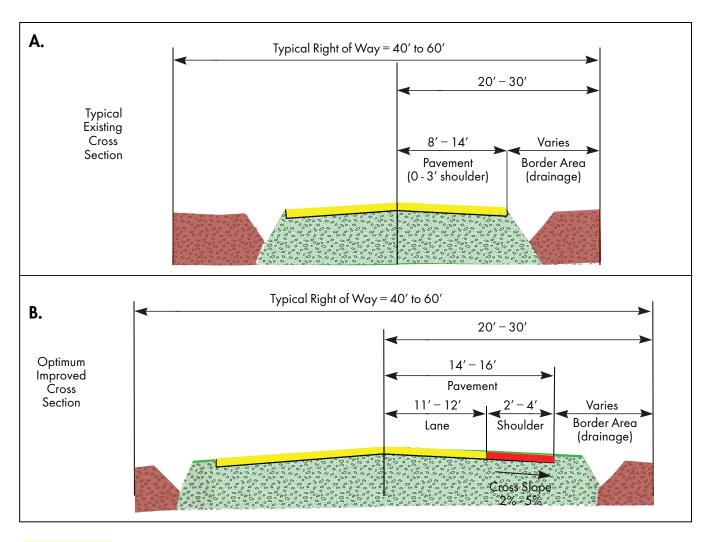
**Figure 7-20:** Rural Road Cross Section on Constrained Right of Way
