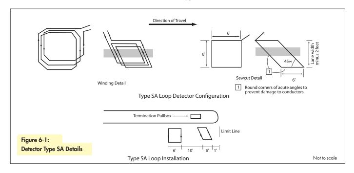
Figure 6-1 (left) illustrates Detector Type SA used by the City of Cupertino and Figure 6-2 (below) illustrates the typical detector placement at a five-phase signalized intersection
