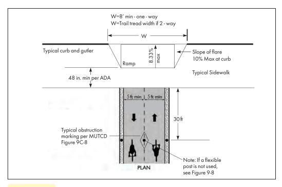
Figure 9-9: Optimal Bollard Layout and Ramp Design
