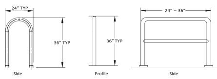
Figure 10-1: Typical Dimensions – Inverted U and Variations
