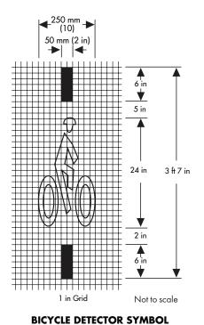
Figure 7-9: **Loop Detector Pavement Marking** (Calrans Standard Plans A24C)
