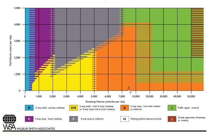
Figure 9-4: **Guidelines for Traffic Control Devices at Trail Intersections**
