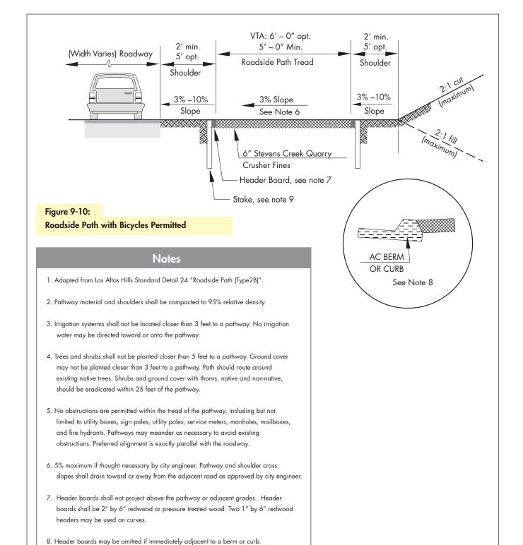
9. Stakes shall be 2" by 4" and 2' long at 6' maximum spacing and at each splice. Connect stake to header with a minimum of 4-10d galvanized nails.
