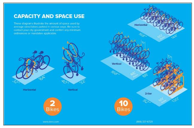
Figure 10-5: Capacity and space needed for typical bicycles
