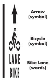
Figure 7-3: **Optimal Bike Lane Pavement Marking Set**
