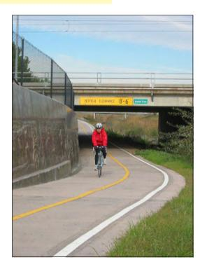
This cyclist has no margin of error on his right, and would benefit from an edge line on both sides. Although low, the bridge is higher than the minimal required vertical clearance of 8 feet.
