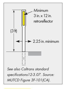
Figure 9-7: Preferred Bollard Design -Flexible Post Channelizer
