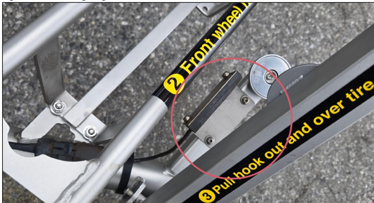
Figure 3-12. Missing Magnet on Bike Rack Retention Arm
