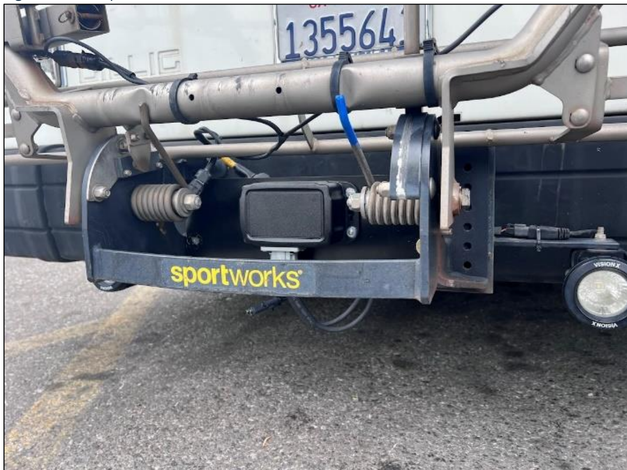
Figure 3-10. Preproduction Velolink Unit Installed on VTA Bus 4403
