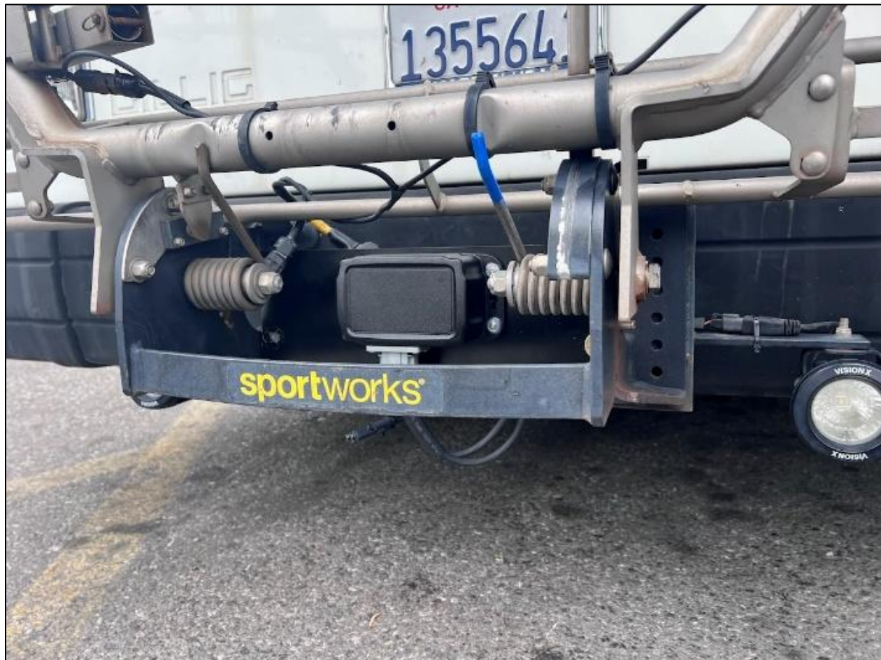
Figure 3-10. Preproduction Velolink Unit Installed on VTA Bus 4403
