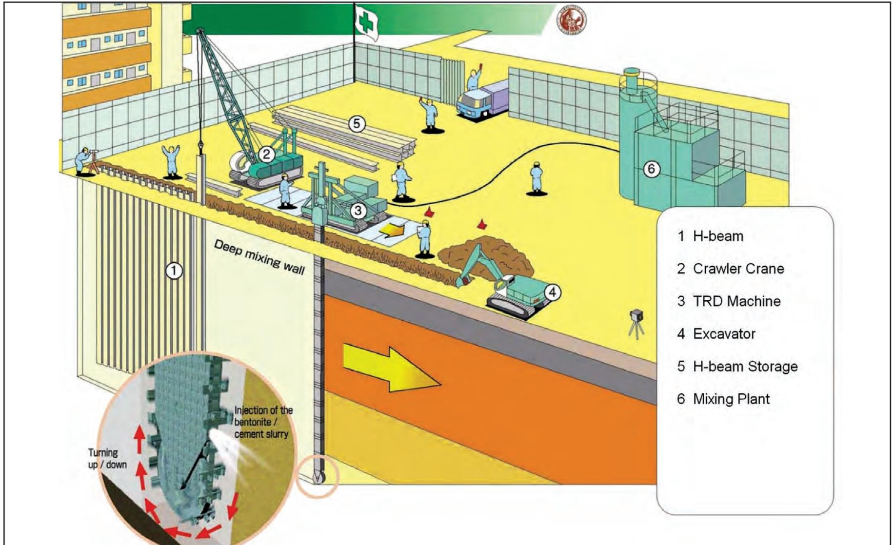
Figure 6-18: Trench Remixing and Deep-Wall Method (TRD)
