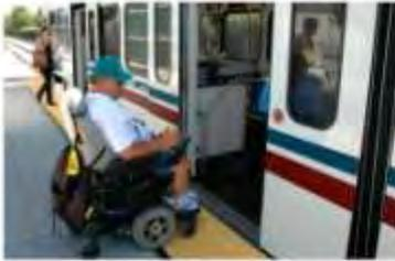
Low-floor light rail vehicles and retrofitted platforms provide quick, level boarding for all riders.
