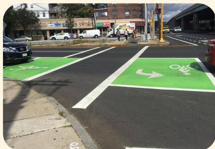
Bike boxes provide a delineated location for bicyclists to wait prior to making a left turning movement, while also signaling to vehicles the upcoming movements of the bicyclists.
