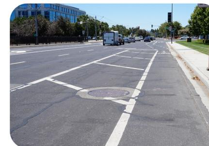
Buffered bike lanes visually delineate a separation between vehicles and bicycles.
