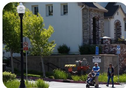
Pedestrian-scale lighting is used to enhance the pedestrian realm and light the travelway of pedestrians.
