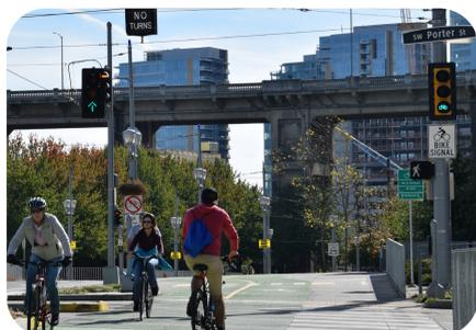
Bike signals are used at signalized intersections to facilitate bike crossings through the intersection.
