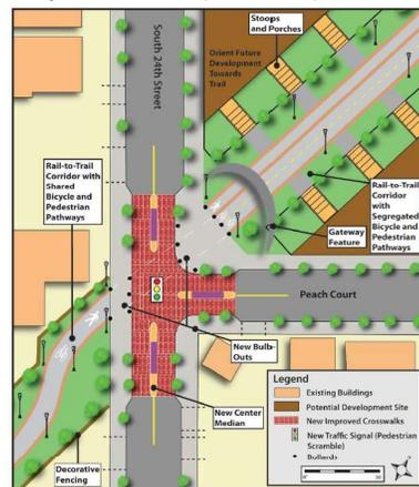
Figure 53. Rail-to-Trail corridor Detail Plan D.
