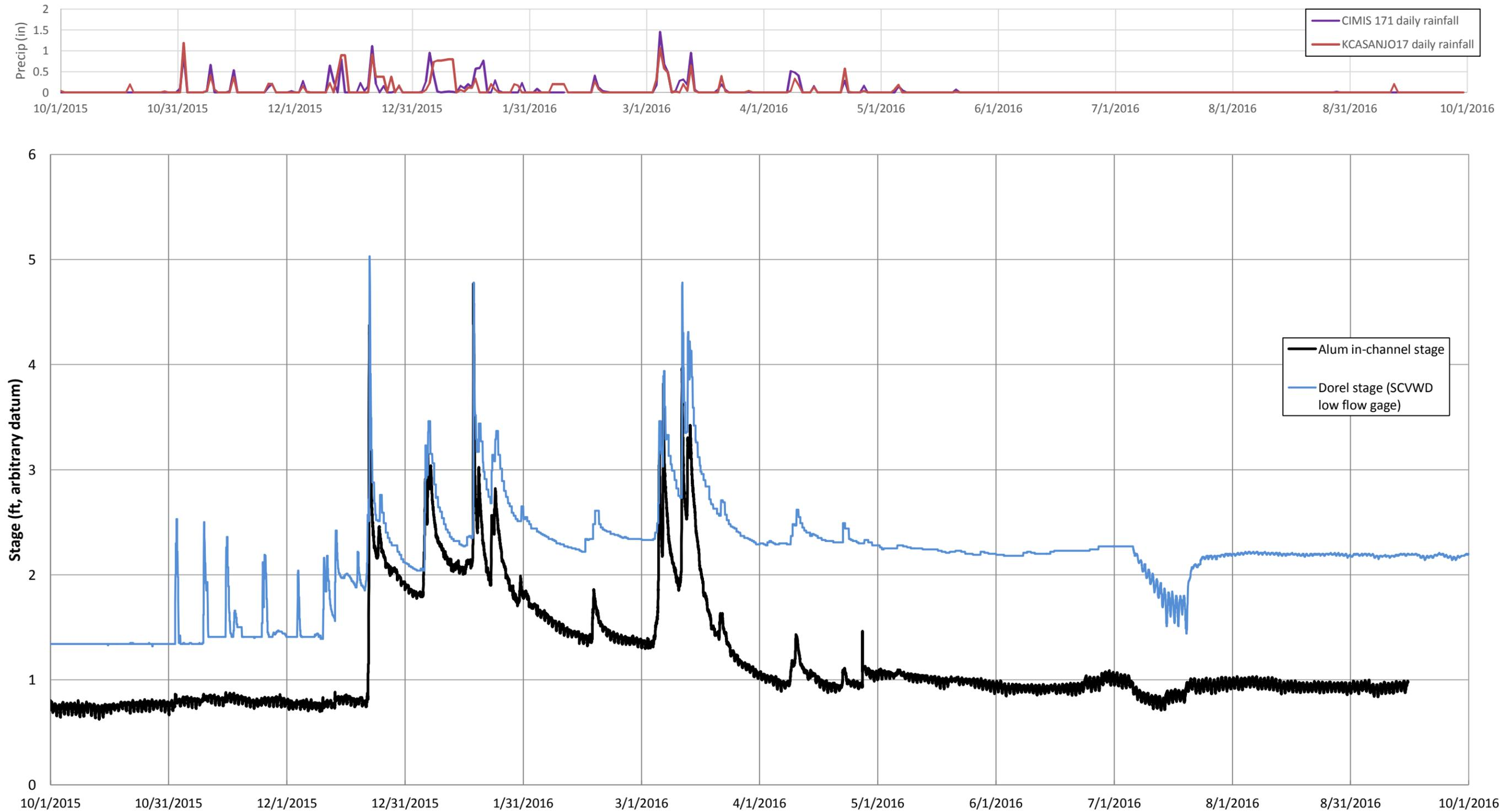
**Figure 5 . Alum Rock 15 minute stage record from upstream channel-bottom pressure transducer, WY2015, Alum Rock monitoring, Santa Clara County, California.** Red squares mark manual readings from the upstream staff plate. These data are compared with hourly stage data from the Dorel gage, located approximately 2.5 km downstream from project sites 10 and 13. Precipitation from nearby gages (KCASANJ17, CIMIS171) are shown above.
