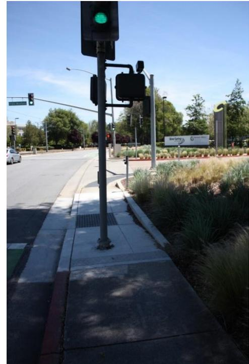
Photo 8: Traffic signal blocking the sidewalk on at Vista Montana
