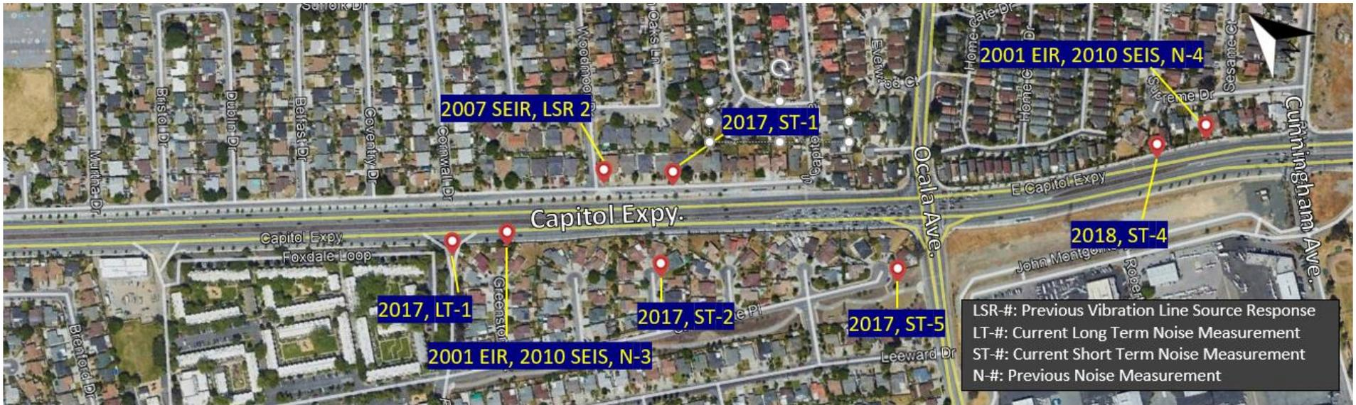
**Figure 3: EBRC Project Area from STA 1003+00 to STA 1050+00. Current and Previous Existing Noise and Vibration Propagation Measurements Indicated**
