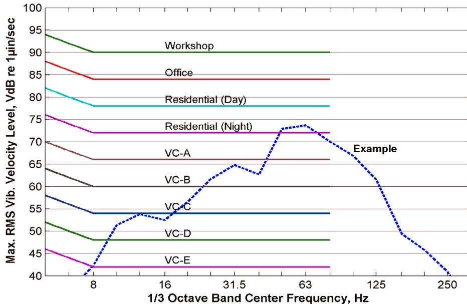
**Figure 5: FTA Detailed Vibration Analysis Criteria**
