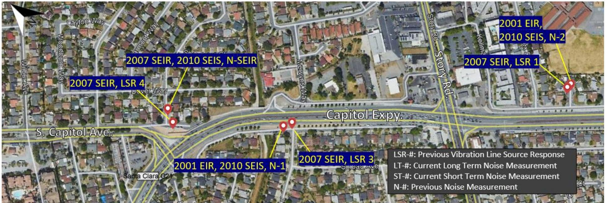
**Figure 2: EBRC Project Area from STA 965+00 to STA 1003+00. Current and Previous Existing Noise and Vibration Propagation Measurements Indicated**
