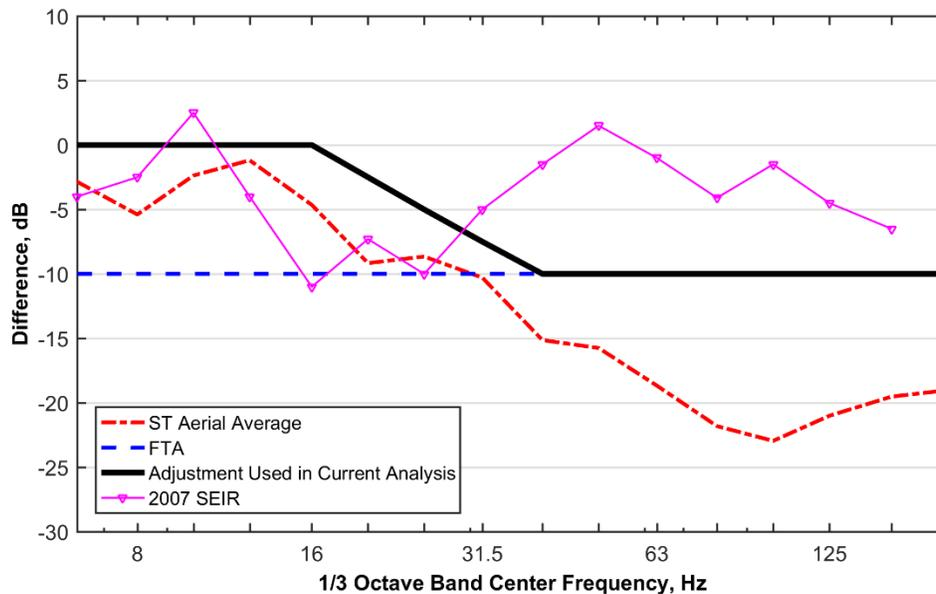
**Figure 8: Ballasted Track to Aerial Structure Adjustment Factor**
