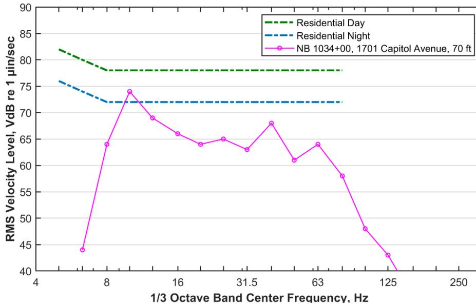
Figure 10: Estimated Vibration Spectrum for Receiver NB 1034+00, 70 ft.
