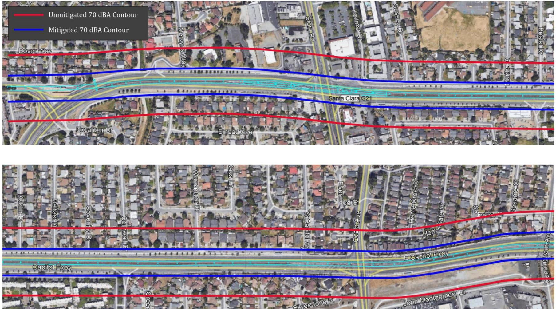
**Figure 14: FTA Nighttime Construction Noise Criteria Contours for Unmitigated and Mitigated (10-foot Noise Wall) Cases.**
