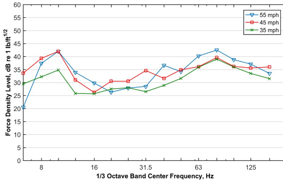
**Figure 7: Ballasted Track FDL: VTA Kinkisharyo (SEIR 2007)**
