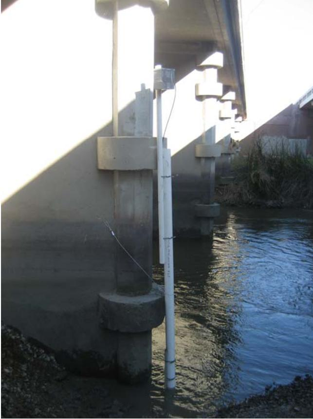
**Photo B-1.** Water-level datasonde installed during a low tide on the Guadalupe River.
