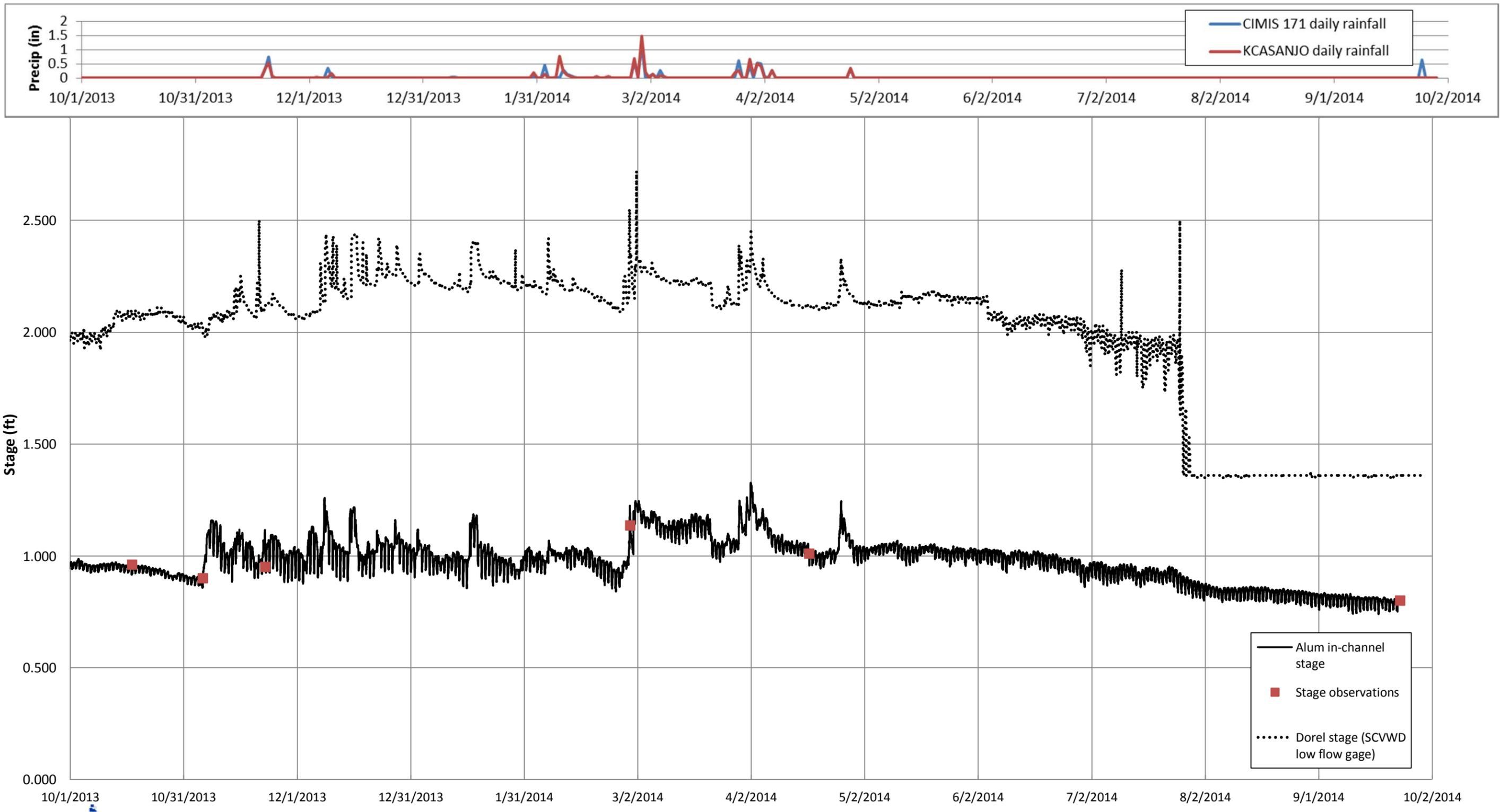
**Figure 5 . Alum Rock 15 minute stage record from upstream channel-bottom pressure transducer (solid line), Alum Rock monitoring, Santa Clara County, California.** Red squares mark manual readings from the upstream staff plate. These data are compared with hourly stage data from the Dorel gage (dashed line), located approximately 2.5 km downstream from project sites 10 and 13. Precipitation from nearby gages (KCASANJ17, CIMUS171 are shown above).
