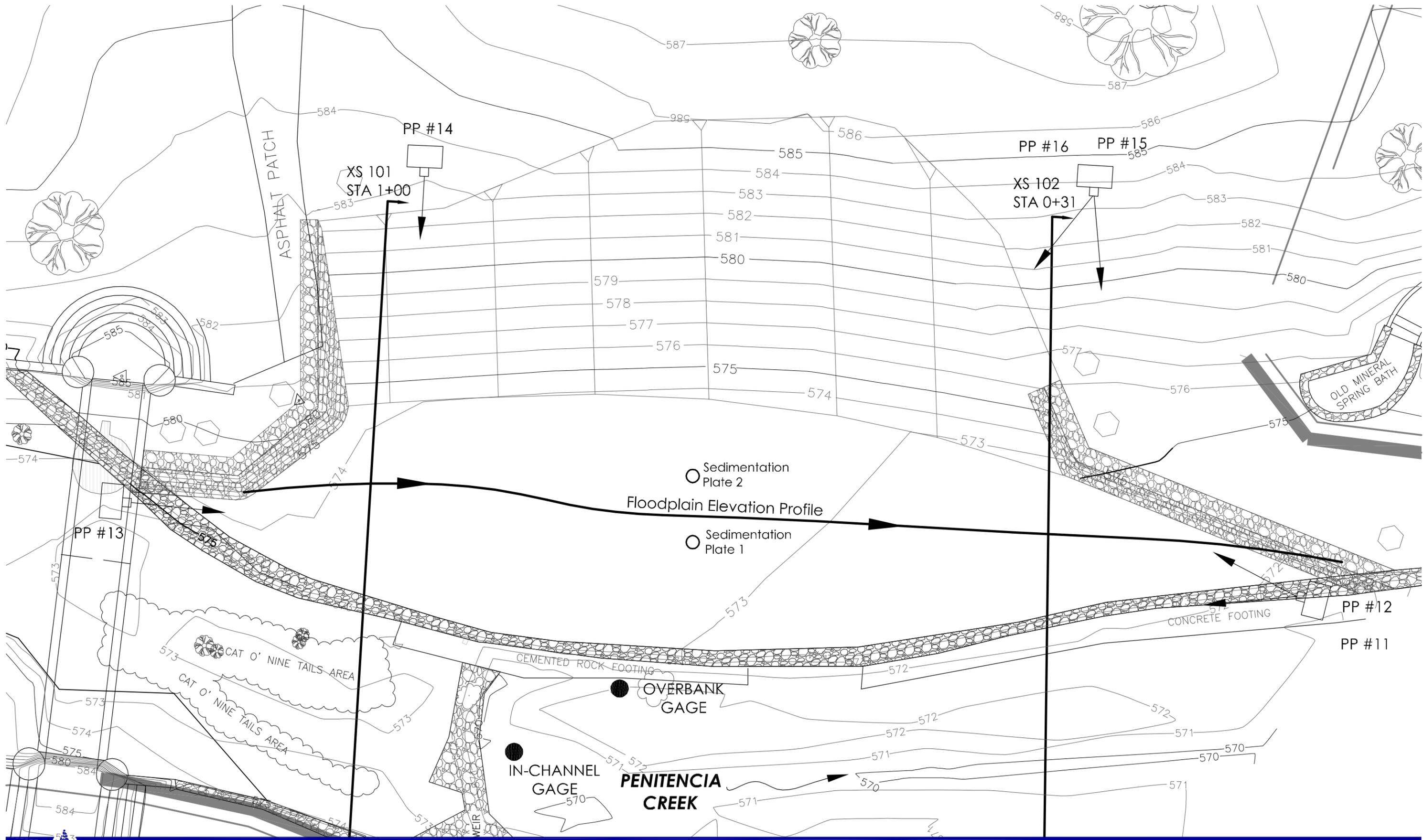
Figure 2. Upper Penitencia Creek, Alum Rock Monitoring, Santa Clara County, California. Project Site 10, a 120-foot long, 30-40 foot wide newly constructed floodplain.
