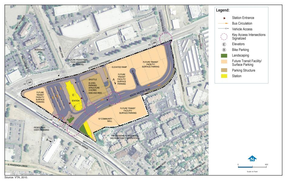
Figure D-2: Milpitas Station Conceptual Site Plan
