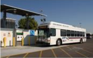
Zero-Emission Bus (ZEB) at hydrogen fueling station
