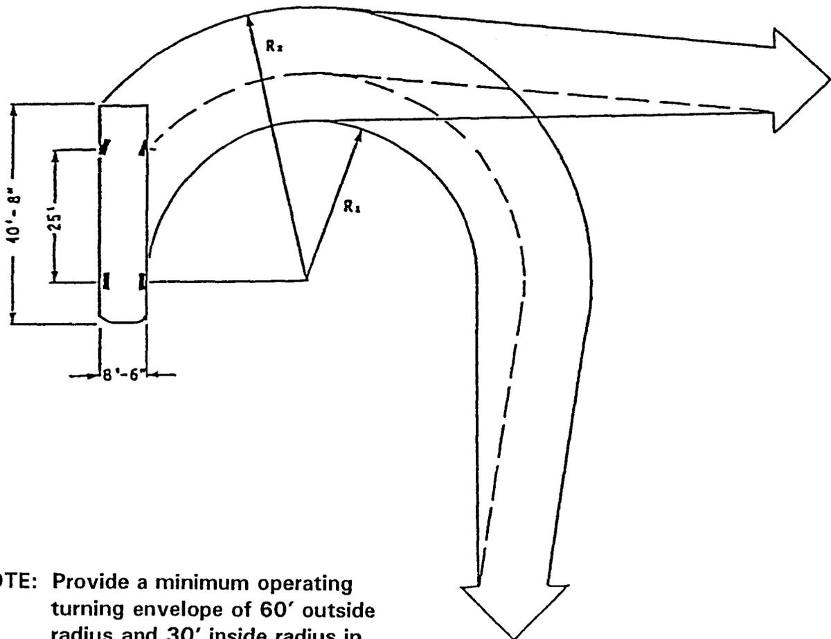
NOTE: Provide a minimum operating turning envelope of 60' outside radius and 30' inside radius in designing the transit centers.
