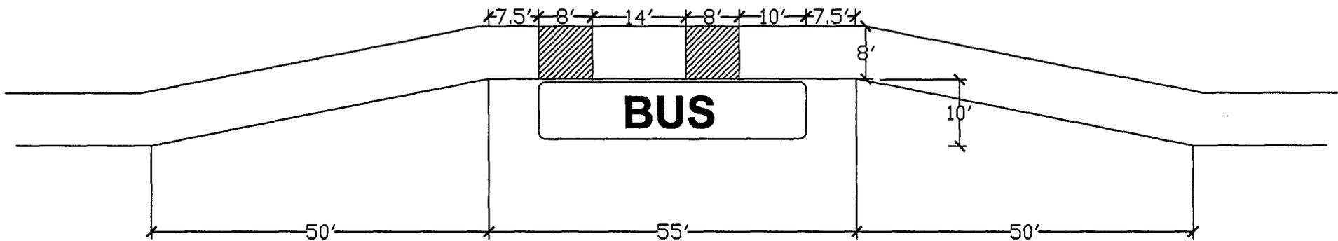
SHADED AREAS SHOWN ON SIDEWALK ADJACENT TO THE BUS STOP SHALL BE CLEAR OF ANY PHYSICAL OBSTRUCTIONS.
