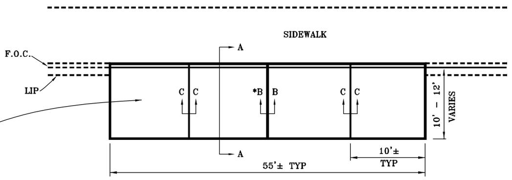
SAWCUT AND EXCAVATE EXISTING PAVEMENT, INCLUDING CURB & GUTTER. REPLACE WITH P.C.C. PAVEMENT SECTION AND MONOLITHIC CURB.
